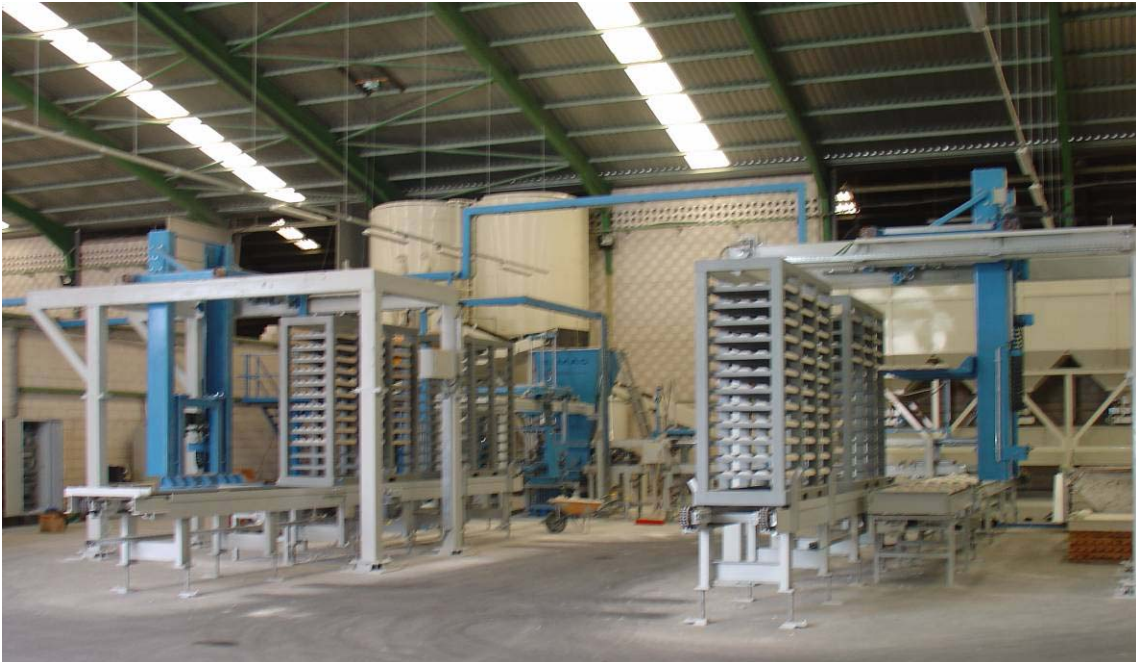
RAC Mobile Racking System for RFS Flat Stack; for e.g. 3 x 10 pallets per fork lift ride
